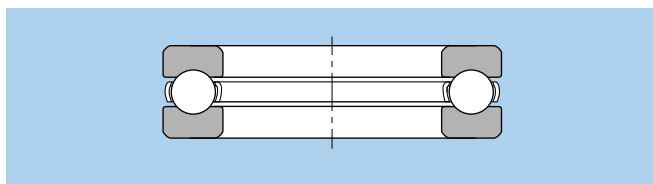
Fig.1 Single type thrust ball bearing (Example of the press cage)
