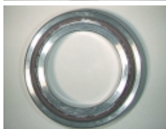
Photo. 6.1 Filling grease into angular contact ball bearing
