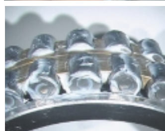
Photo. 6.2 Filling grease into cylindrical roller bearing
