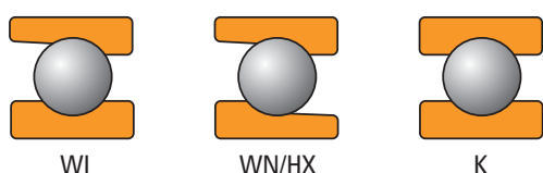
Fig. 21. Angular contact spindle bearing types.
